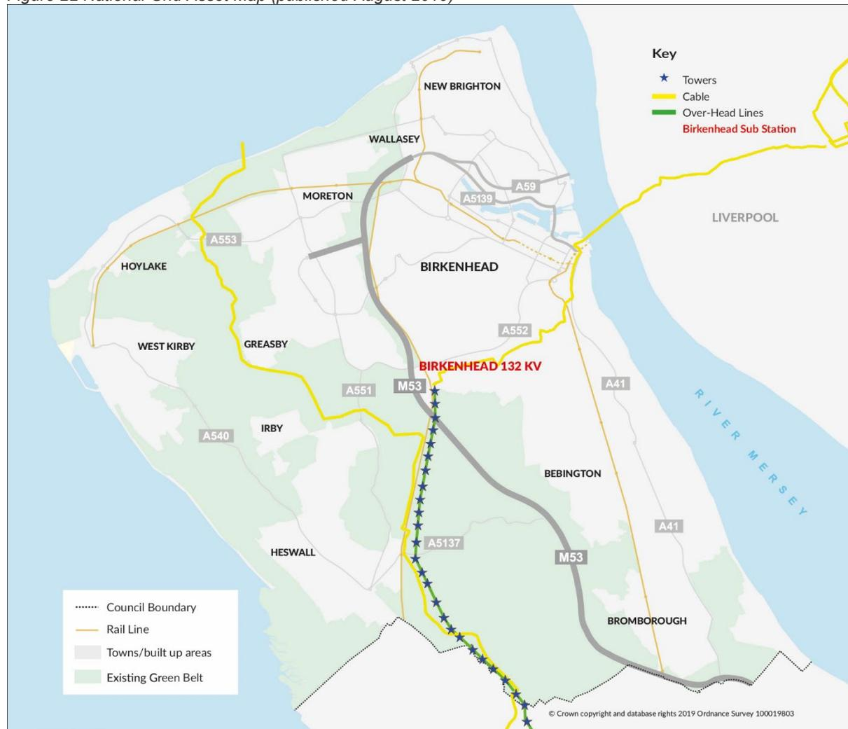
91. The majority of the Borough's electricity is provided via National Grid's high voltage electricity overhead transmission 275kV line from Capenhurst and underground cables from Liverpool to Prenton, as shown in Figure 22. Energy generated by the wind farms in Liverpool Bay also connects to the grid at Birkenhead. A trans-national high-voltage cable from Scotland, via the Irish Sea and Liverpool Bay, to Meols and Connah's Quay was also completed in 2018.
