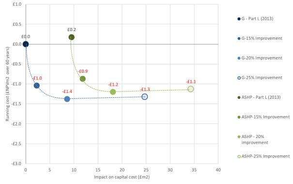
Figure 6.10 Relative running and capital costs for an air-conditioned office with different heating systems and space heating demand in 2025
