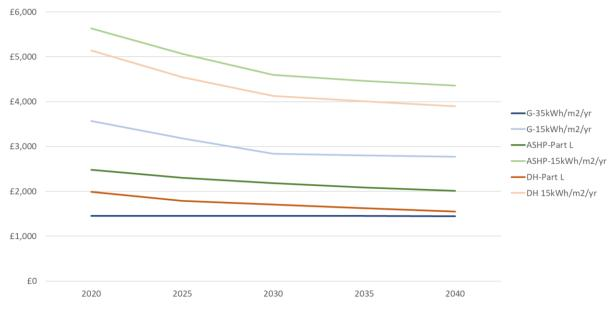
Figure 5.6 Projected trend in the additional capital costs of building to higher standards overtime – semi detached house
