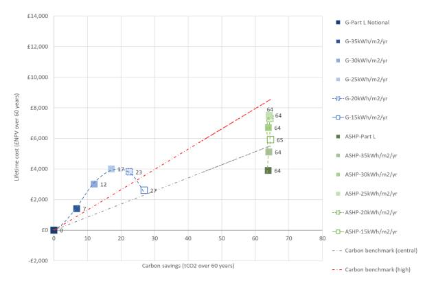
Figure 5.13 Carbon savings and lifetime costs of semi-detached house with different heating systems and space heating demand in 2025
