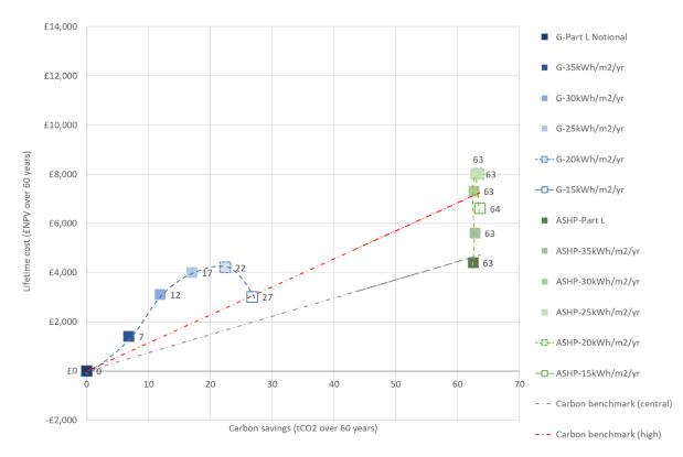
Figure 5.12 Carbon savings and lifetime costs of semi-detached house with different heating systems and space heating demand in 2021
