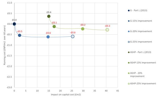
Figure 6.8 Relative running and capital costs for a naturally ventilated office with different heating systems and space heating demand in 2025
