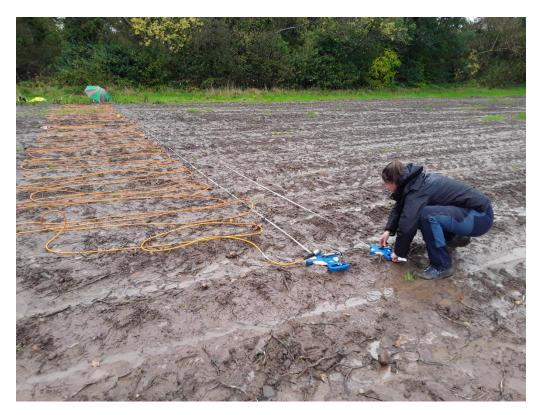
Figure 3 – Electrode Array
