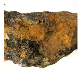
Several other examples of evidence of iron smelting have been recovered, from heavy iron rich tap slag to frothy high silicate/ash slags.
