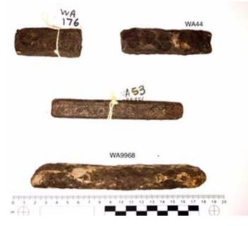
**WA9968** Iron bar 150mm in length and c. 28 x 15mm in section. There is a slight curve to the bar so as to describe an arc. The outer edge being rounded, the inside edge is square.
