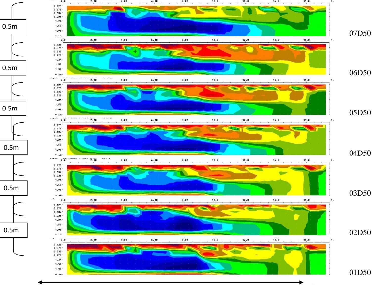
[locational data removed] – Schlumberger - 36 Electrodes @ 0.5m spacings – Lines @ 0.5m spacing
