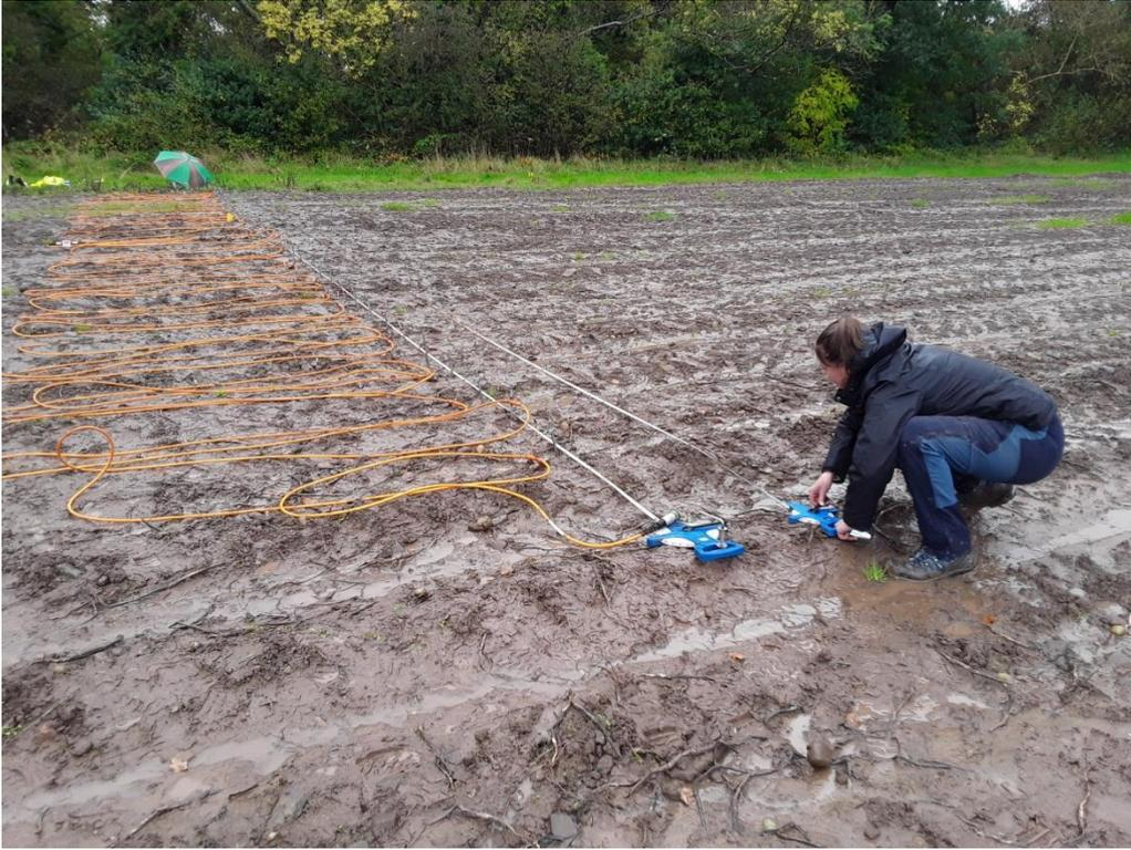
Figure 3 – Electrode Array
