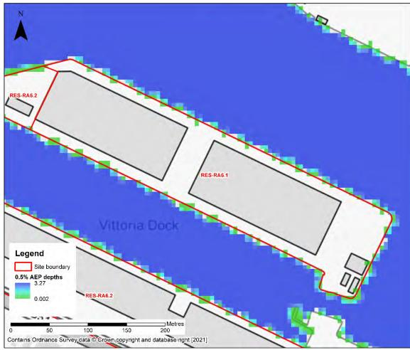
Figure 3: modelled tidal flood depths (m) for 0.5% AEP baseline event
