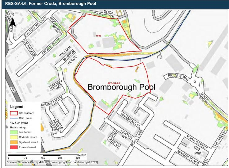
Figure 8: 1% AEP event surface water flood hazards (Risk of Flooding from Surface Water map)
