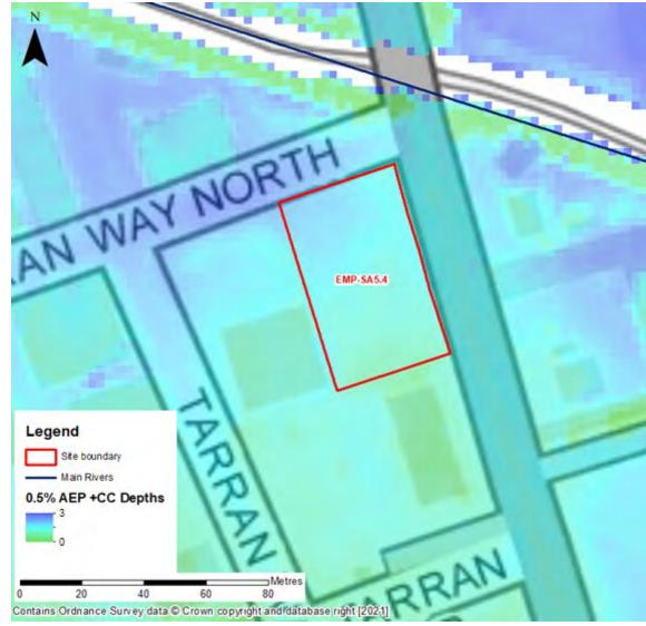
Figure 9: modelled tidal depth for the 0.5% AEP plus climate change breach scenario of the Wallasey Embankment
