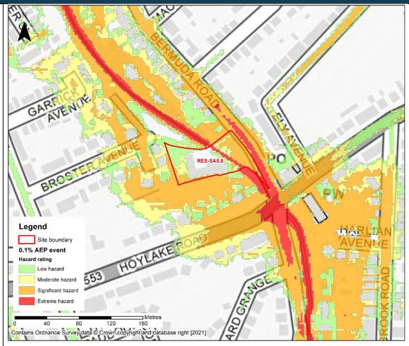
Figure 9: 0.1% AEP event surface water flood hazard (Risk of Flooding from Surface Water map)
