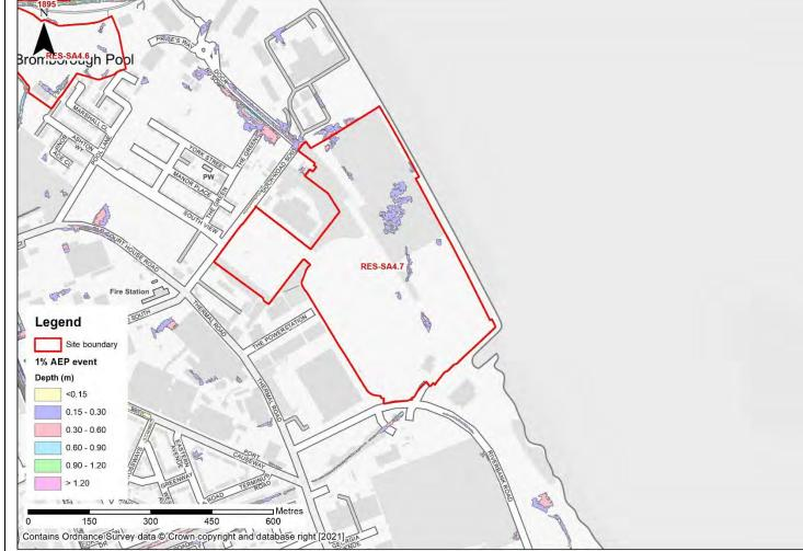
Figure 8: 1% AEP event surface water flood depths (Risk of Flooding from Surface Water map)
