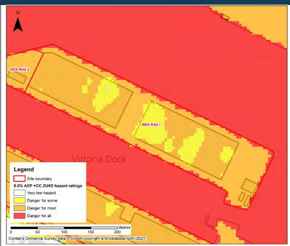
Figure 7: modelled tidal flood hazard for 0.5% AEP +climate change event
