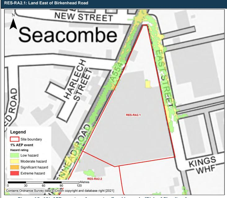
Figure 10: 1% AEP event surface water flood hazards (Risk of Flooding from Surface Water map)
