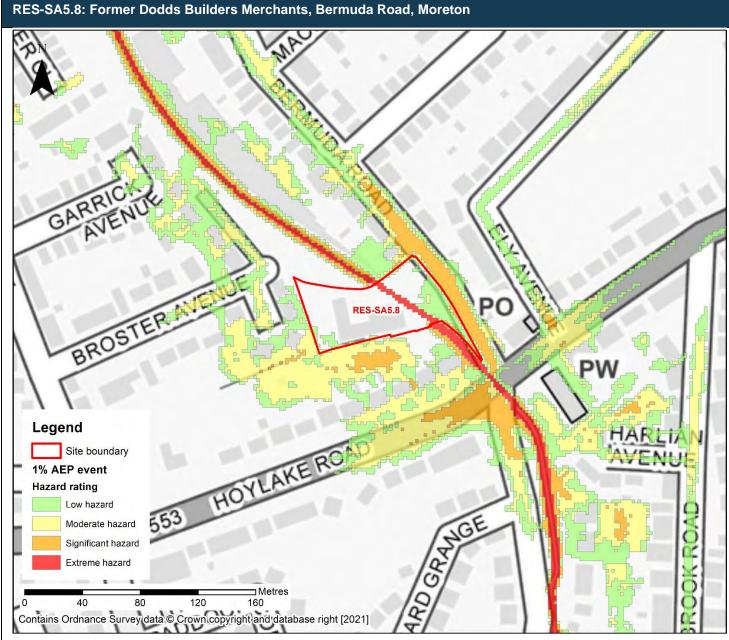
Figure 7: 1% AEP event surface water flood hazards (Risk of Flooding from Surface Water map)
