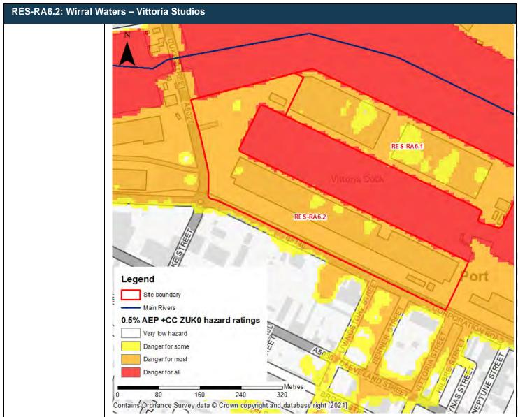
Figure 7: modelled tidal flood hazard for 0.5% AEP +climate change event  $\,$
