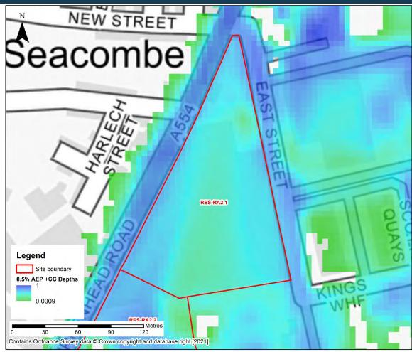
Figure 5: modelled tidal flood depths for 0.5% AEP + climate change event
