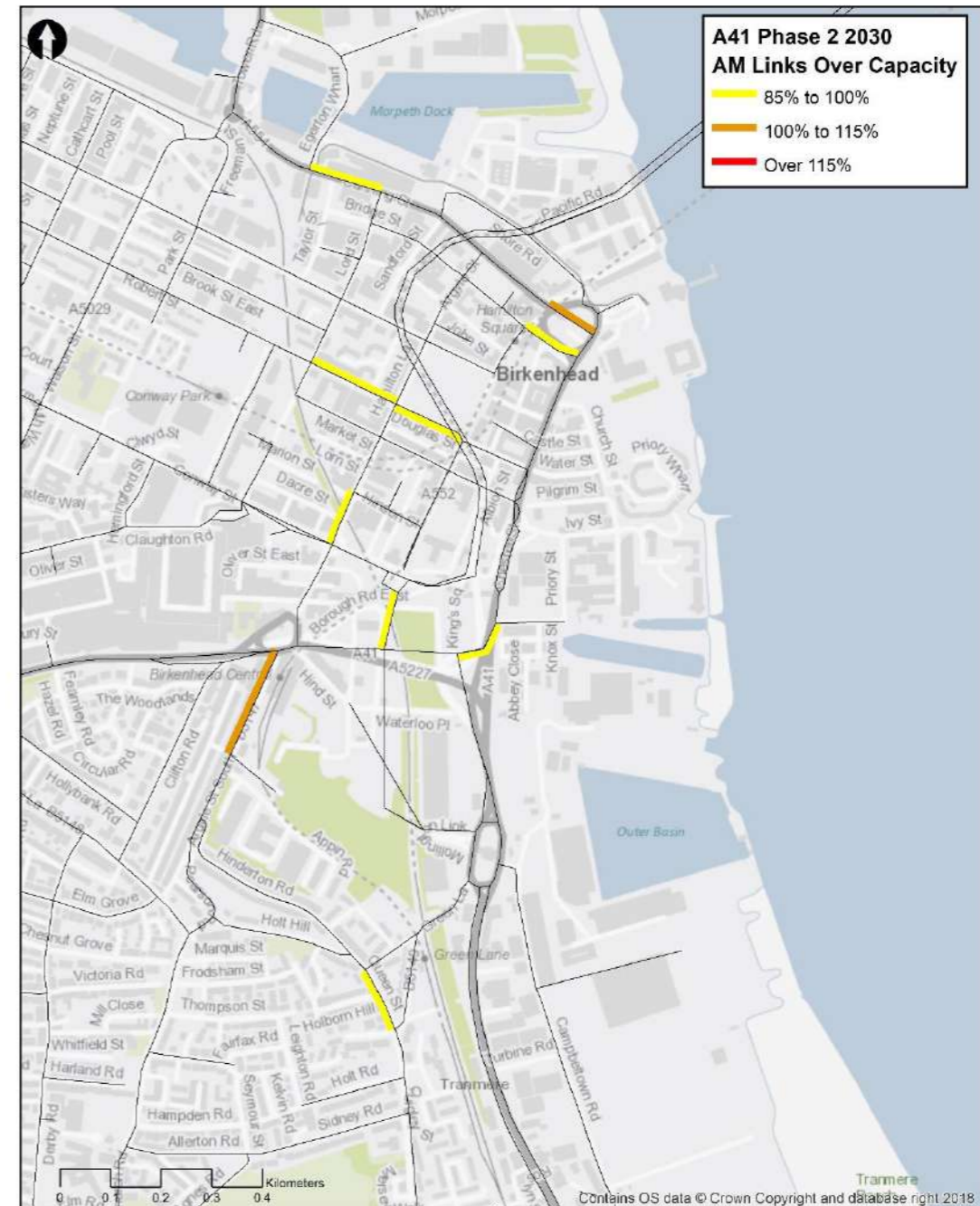
Figure 19: A41 Phase 2 2030 AM Links Over Capacity
