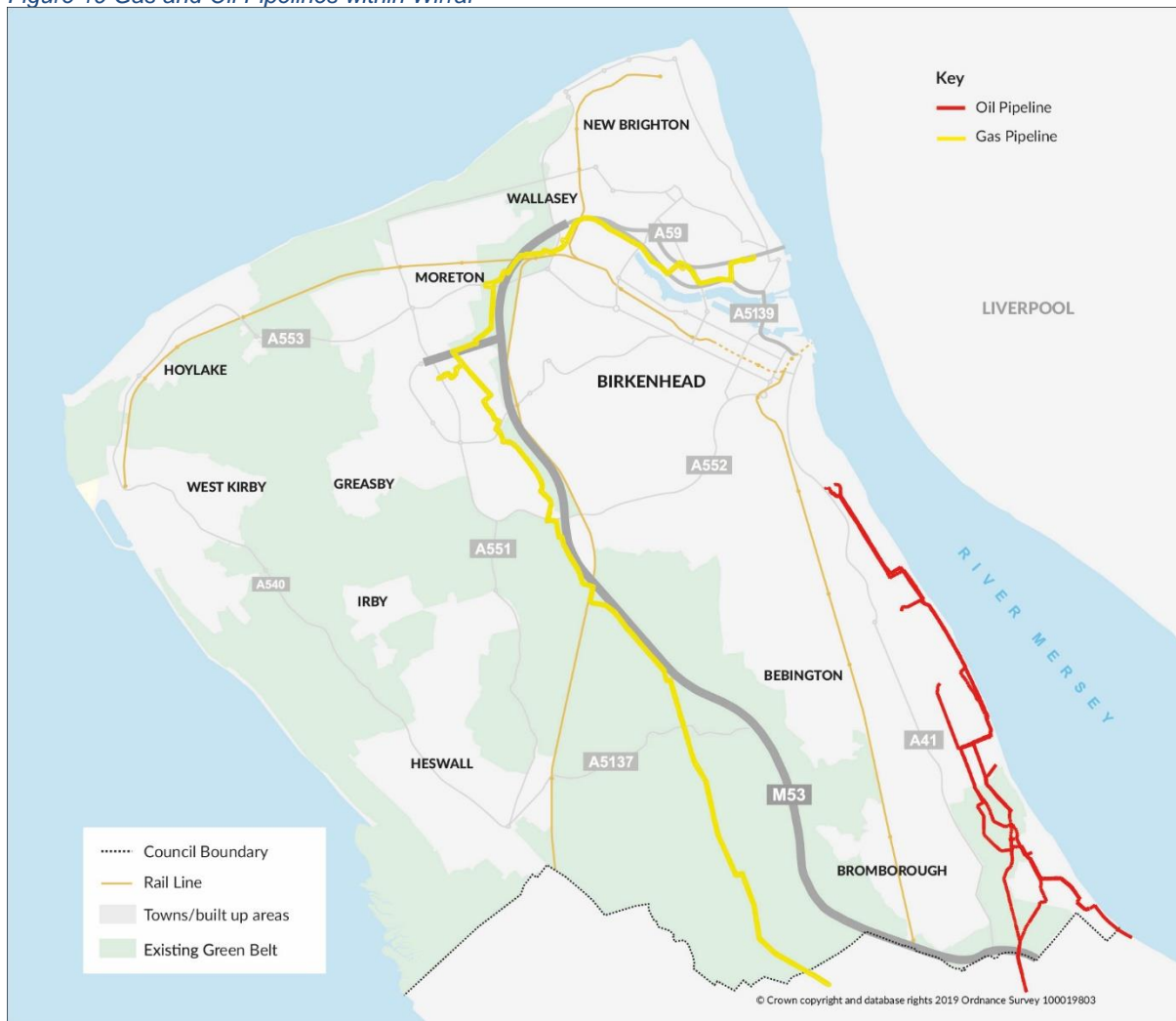
Figure 19 Gas and Oil Pipelines within Wirral
