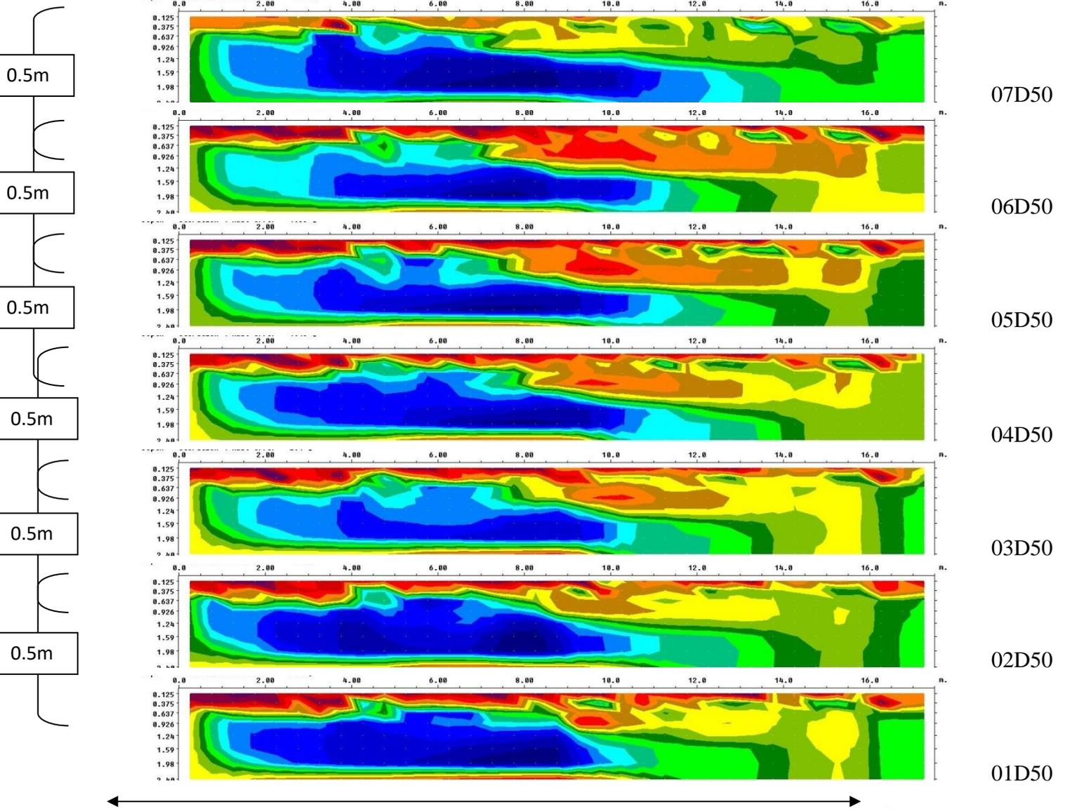
[locational data removed] – Schlumberger - 36 Electrodes @ 0.5m spacings – Lines @ 0.5m spacing
