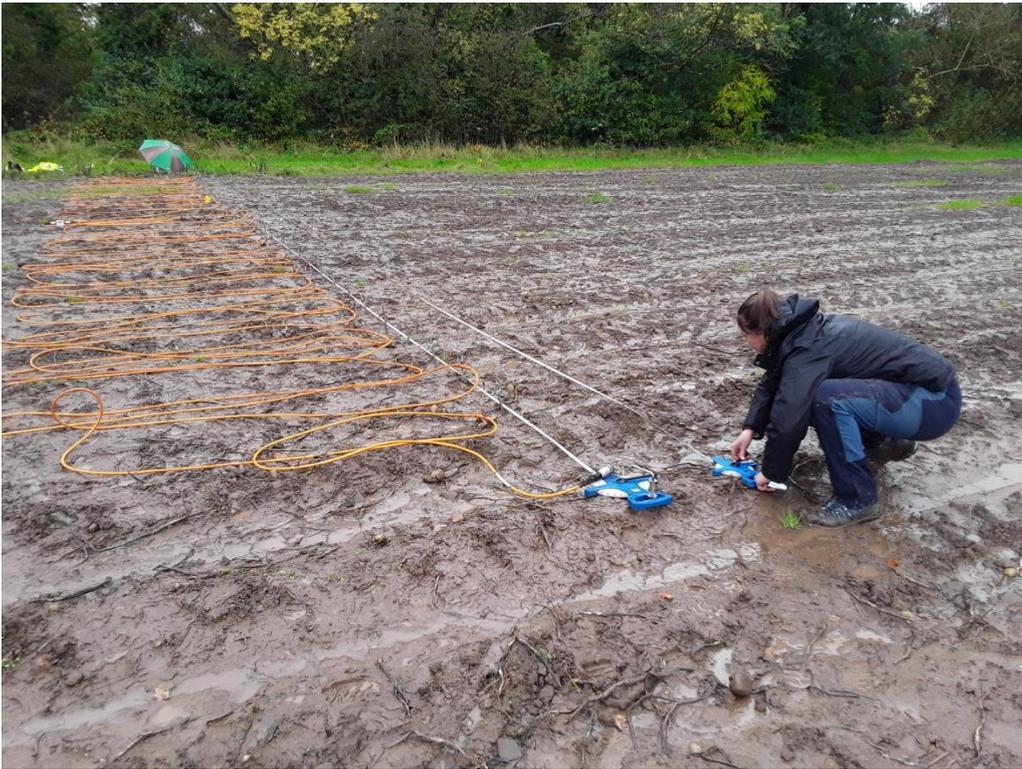
Figure 3 – Electrode Array
